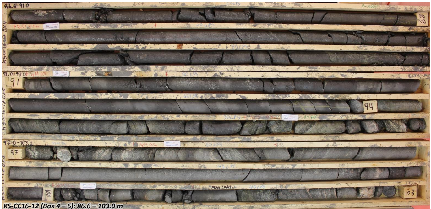
Figure 5: Core photo of drillhole KS-CC16-12 showing part of the graphitic fault intersected at the Loki Zone between 86.6 – 103.0 m in boxes 4 - 6.
